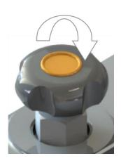
3) ③ Turn Vent / Release valve to CW to close the Vent / Release valve.
