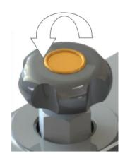
7) When calibrating while depressurize, open the vent valve very slowly to see that the pressure decreases, close the vent valve when it reaches the target pressure, and adjust the pressure again using 6 Fine Pressure Adjustment.
