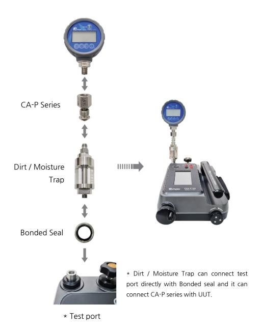
1-1) For UUTs suspected to be contaminated, connect UUT, CA-P, Dirt / moisture trap, bonded seal and test port (1/8" PF) in order.
