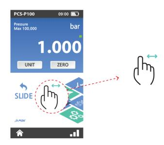
To measure electrical signals from the pressure transmitter and power the transmitter, slide your finger to the lower screen and slide to the right to move the screen with a "click" sound (relay working). Change the order of the screens as shown below. The content is explained in Chapter 2.4.
