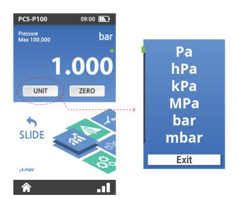
Touch and scroll to change units Pa  $\rightarrow$  hPa  $\rightarrow$  kPa  $\rightarrow$  MPa  $\rightarrow$  bar  $\rightarrow$  mbar  $\rightarrow$  kg/cm<sup>2</sup>  $\rightarrow$  psi  $\rightarrow$  mmH<sub>2</sub>0  $\rightarrow$  mH<sub>2</sub>0  $\rightarrow$  inH<sub>2</sub>0  $\rightarrow$  mmHg  $\rightarrow$  inHg.
