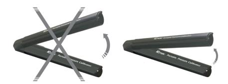
5) ④ Generate the target pressure (Vacuum) with Hand pump Pressing the pump up once without volume will apply a lot of Vacuum. Short stroke will generate small Vacuum.
