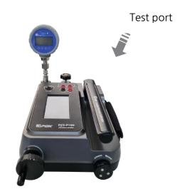
\* Test port is 1/8" PF Female and it connected 1/4" Lok Male. 1/4: Lok Male can connect CA-P series. 1/4" Lok Male fitting can be separable from 1/8" PF Female.
