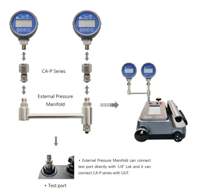
1-2) When calibrating two UUTs of the same range at the same time, use External pressure manifold.
